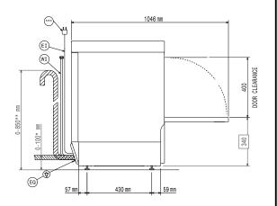
\* Without drain pump \*\* With drain pump \*\*\*Plug only for Single Phase Machine
